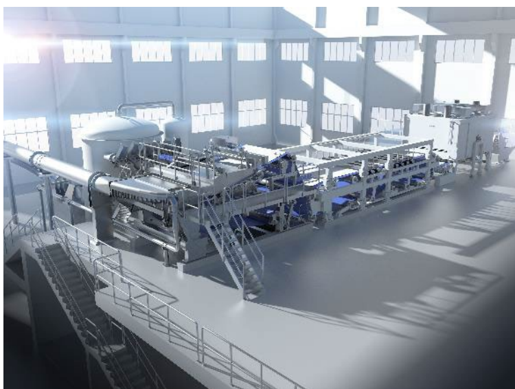
ANDRITZ neXline wetlace line for the production of flushable wipes
